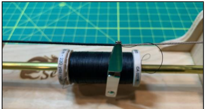
Adding a small handle to the right hand crank made it easier to operate the unit.
